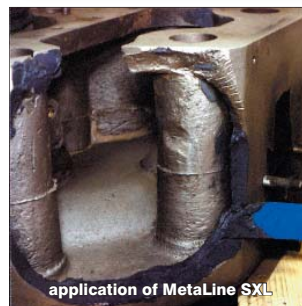
casing breakage at a cylinder head
