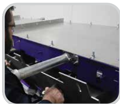
Externally replaceable liners for easy maintenance
